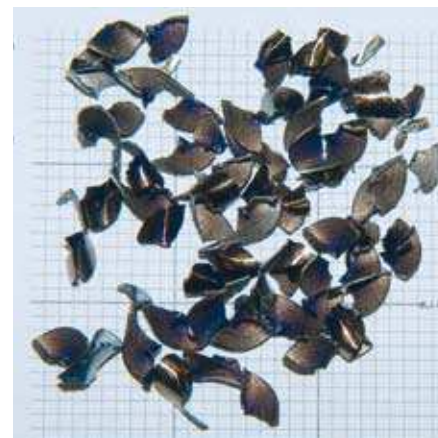
Fig. 3: Problem-free chips preventing chip congestion and jamming of the tool.
