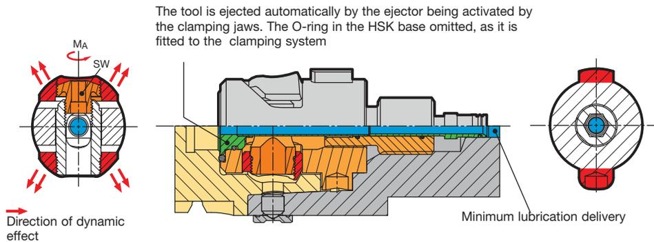
Bending, torsional and tightening moment for 4-point clamping sets for MQL
