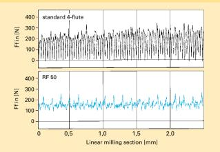
A cutting force comparison between a conventional type N and a RF 50 variable helix end mill clearly shows the RF 50 end mill's quieter and more stable machining characteristics.
