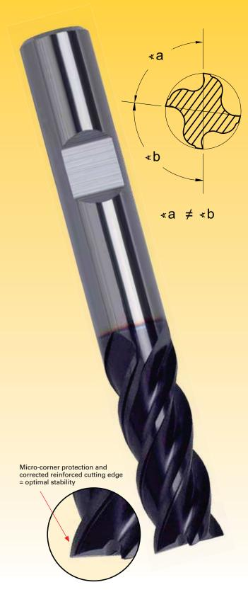
We have developed the RF 50 end mill with variable flute spacing primarily to prevent chatter and the so-called corkscrew effect (as found when withdrawing tools having a large spiral angle)
