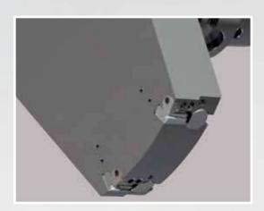
Application: Face milling of a valve plate on a MC, complete coverage required
