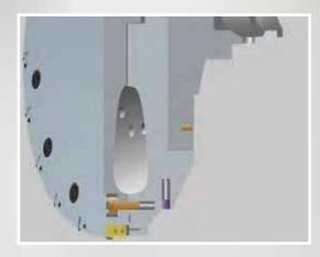
Application: Face milling of a valve plate on a special purpose machine
