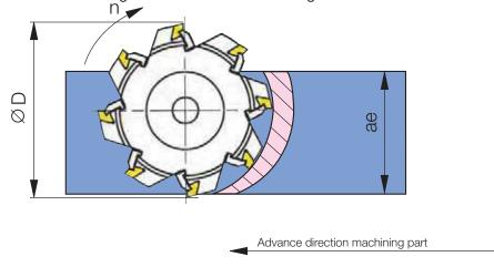
Insufficient clamping of the workpiece, an extreme tool overhang as well as the wrong choice of cutting parameter directly influence the miling results as well as the surface quality, tool life and processing time is concerned.
