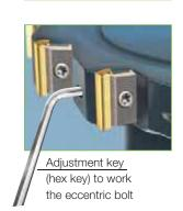
**Security advice:** For security reasons the milling cutter must be returned to the manufacturer for inspection if the holder is damaged! The clamping sets must be renewed on a regular basis or in case that they show any sign of damage. Only original spare parts may be used!
